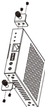
**Step 2:** Insert the product with mounting ears into a 4U rack (up to 12 units can be installed vertically), as shown in the figure below:
