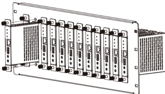
**Step 3:** Use screws to fix mounting ears on the rack to complete the mounting, as shown in the figure below.
