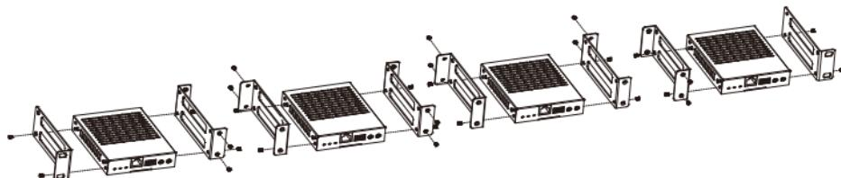
**Step 3:** Fasten screws between two 1U rack panels, so that four products are mounted in a 1U rack, as shown in the figure below.
